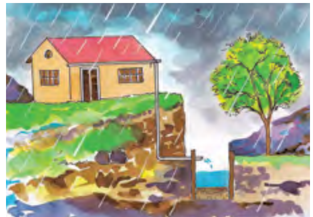
Making rainwater seep into the soil
