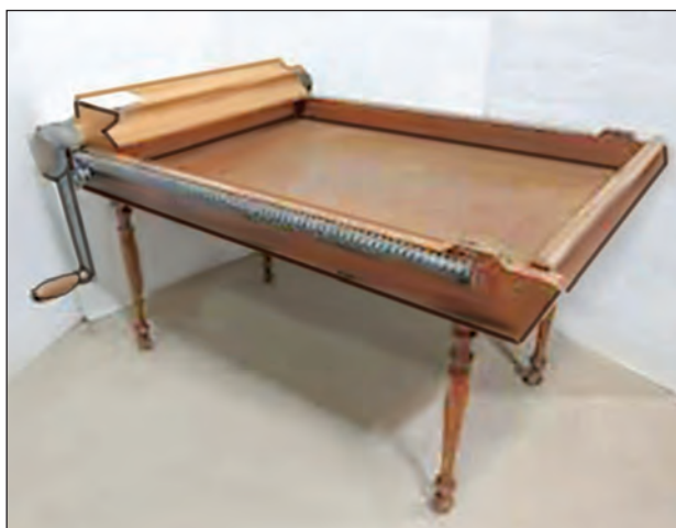
Fig. 10.23 : Wooden Butter worker
