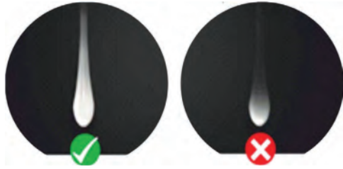
Detection of water in milk
