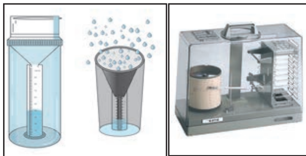
(i) Non recording rain gauge
